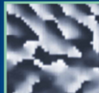
Detail of a grey-level LDW mask for Diffractive Optics. The pixel size is 2 \times 2 \mu\text{m} .
