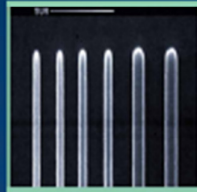
Test pattern on 0.5 \mu\text{m} thick photoresist. The narrowest lines are 0.8 \mu\text{m} wide, with an edge roughness below 0.2 \mu\text{m} .
